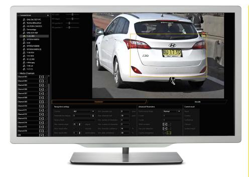
This option enables number plate recognition for license plates from Australia and the USA, among other countries. Additonal countries are available on request. In combination with the Vehicle Access Manager, this enables automatic control of access barriers and gates in car parks, loading zones, property access roads, etc. If a number plate is recognized, the corresponding metadata is linked to the image material and recorded.
