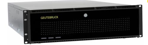
G-Storage is particularly suitable for redundant storage expansion in large to very large video security systems. The high-speed SAS (Serial Attached SCSI with 12 Gb/s) interface makes it possible for G-Storage to handle very large amounts of data without delay, to store it redundantly, and to make it available in milliseconds.
