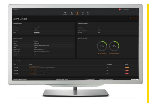
G-Health prevents system failures by a permanent function control. If a critical condition, such as a camera failure or a database error, is detected, the responsible administrators or maintenance technicians immediately receive a corresponding e-mail or a G-Health Alarm in their web interface, stationary or mobile and thus have the possibility to react before a failure occurs.
