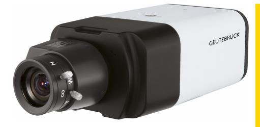
The Box Camera with 4 MP resolution is suitable for indoor use or installation in weatherproof housings. For an ideal adjustment a suitable lens can be freely selected depending on the application. The lens is not included in the scope of delivery.
